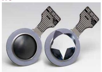
The BS&B Safety Systems ITC rupture disk is specifically designed for protection of intermodal tank containers. The ITC conforms with the latest norms IMO, ADR, RID, US DOT, DOT blue book and ISO. The ITC is a scored tension loaded rupture disk assembly.
