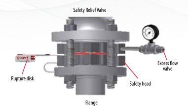
A typical piping arrangement is shown in figure 4. The telltale indicator consists of a pipe nipple, tee, an excess flow (flow check valve), and pressure gauge. The outlet side of the excess flow valve has a threaded connection. If free venting is not desirable, a discharge line can be installed to permit dispersion of product to a safe location.
